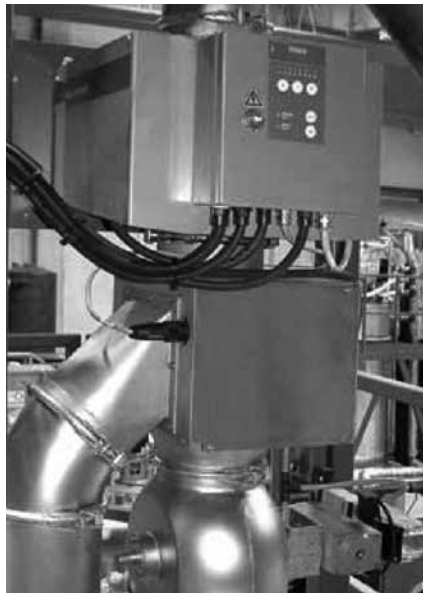
Metal separator MODEL FF used for the quality control of PET regrind
