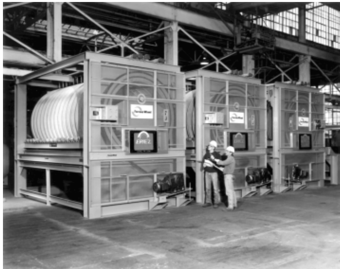
Each of these 15 ring model Ferrous Wheel Separators can process up to 22 tons per hour of iron ore, using only five kilowatts for operation.
