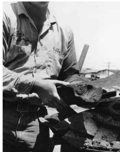
Figure 3. Large Pieces of Tramp Iron Automatically Removed from Processing Line
