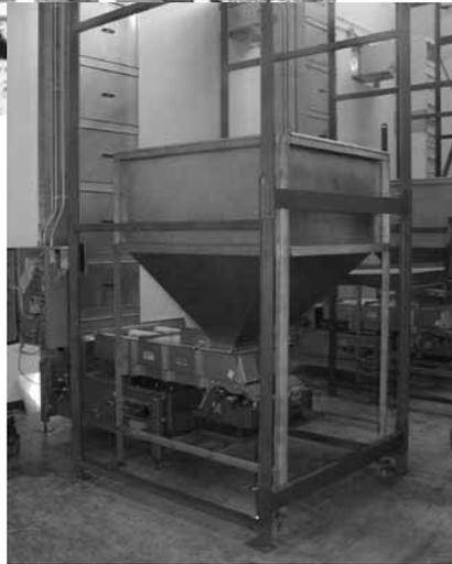
Eriez 56C Tandem Drive feeder metering material from a hopper to a bucket elevator. Consistent feed is required for uniform bucket fill, spillage control and optimum bucket lift performance.
