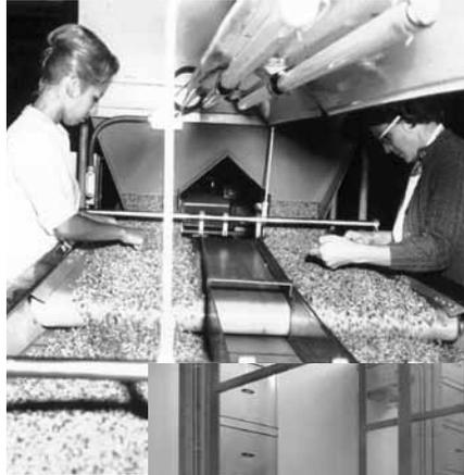
In one of the world's largest walnut processing facilities, all nutmeats are given a rigid final inspection before packaging. This involves use of 40 Eriez Vibratory Feeders to maintain a constant, uniform flow of nutmeats to inspectors at final grading tables.
