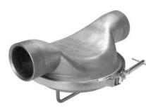
The Model U Trap utilizes a Rare Earth magnet circuit to remove fine and weakly magnetic contamination like rust, scale, or screen wire. Model U Traps remove ferrous contamination from difficult-to-flow or chunky products likevegetables, salsa, or meat batters.
