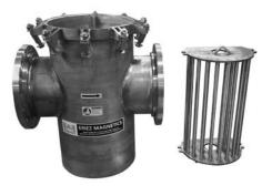
Reduce damage and maintenance to filters, pumps, refiners and other processing machinery handling paper, chemical slurries and other liquid materials. Rugged welded pipe and reinforced plate construction withstands working pressures up to 75 psi (5.3 kg/sq cm). Pressure drop through unit is no more than that of a 90° elbow.
