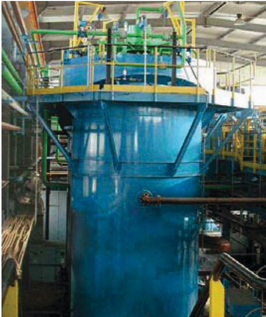
The concentration of minerals by column flotation is a key mineral processing technology. EFD has designed, supplied and commissioned over 800 flotation columns for cleaning, roughing and scavenging duties worldwide.
