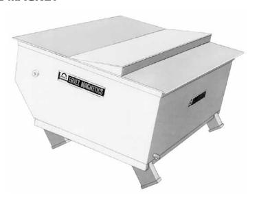
A stainless steel wearplate covers the face of the Eriez Chute–type magnet. Tramp iron collects in the recess below the step so material flow is unimpeded. Installed in chutes inclined up to 60°, these powerful magnets protect valuable machinery by trapping and holding nuts, bolts, knife blades, cutting teeth and other ferrous trash present in fast–moving, entangled sugar cane stalks.
