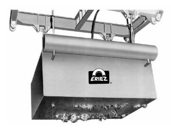
The supporting structure to hold suspended magnets over conveyor belts or feeders can be either stationary or a trolley type so the magnet can be moved away from the processing line to discharge its accumulation of tramp iron. Magnets like this one prevent costly machinery damage, shut—downs and loss of product by removing large amounts of tramp iron each season in sugar mill processing operations.
